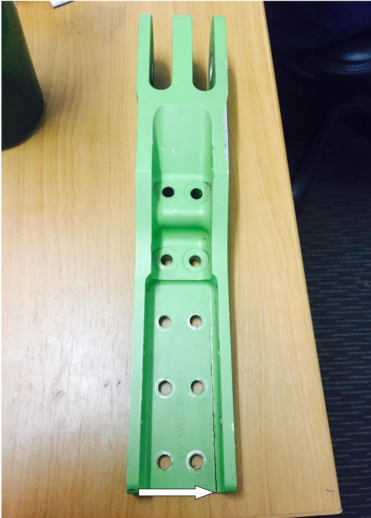
**Figure A – Actual failed fitting showing crack location**
