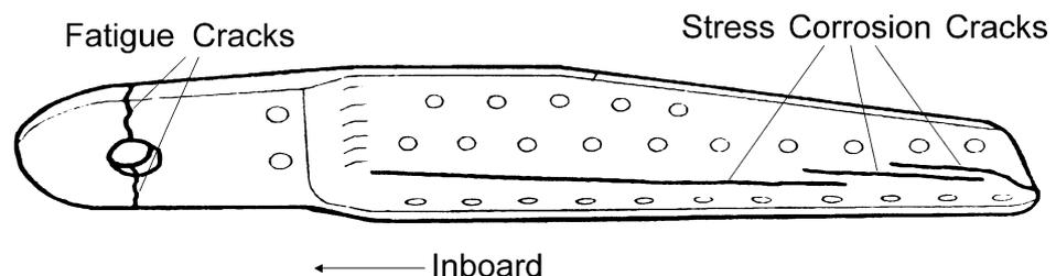
*Note: Fitting shown removed from aircraft (one lug of fitting represented for clarity).*
