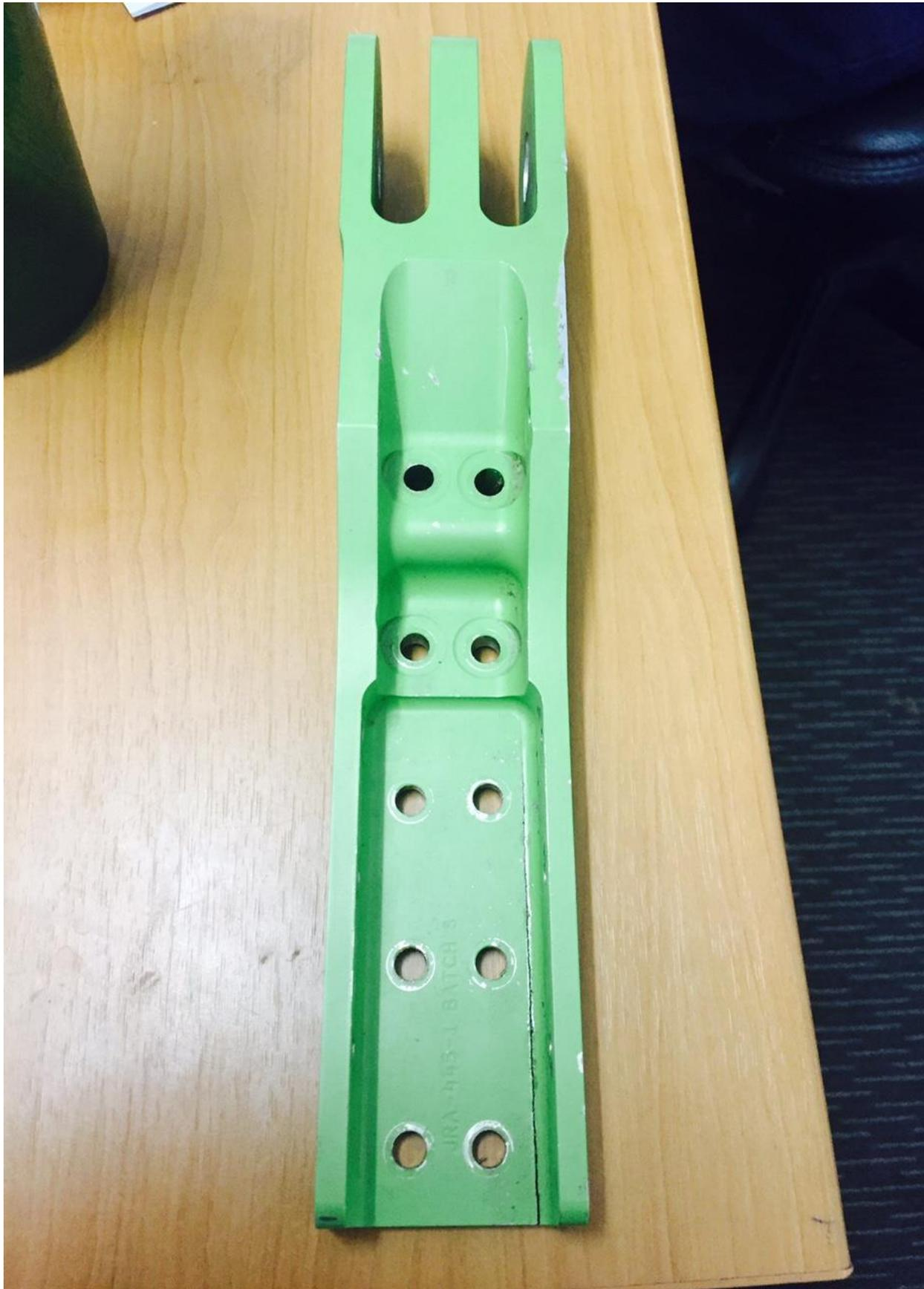
**Figure B – Actual failed fitting showing crack location**
