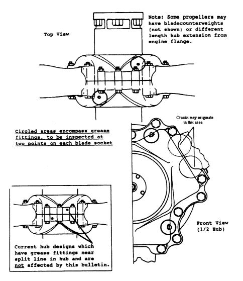
Background: There have been incidents of hub cracks in Hartzell three blade "compact" aluminium hub propellers. Cracks have originated in the threads of a grease fitting hole on the side of the hub and have also originated in the fillet radius area. The cracks are believed to be observable with careful visual examination using a 10X magnifying glass.
