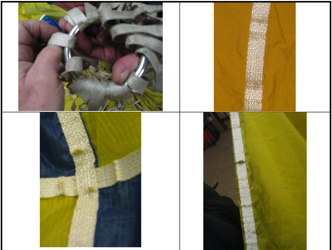
Figure 1: Examples of load tape damage
