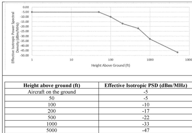
**Figure 2 - Spurious Effective Isotropic PSD at Outside Interface of Airplane Antenna**
