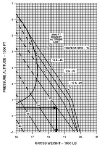
NOTE 1: THIS CHART DEPICTS THE GROSS WEIGHT, PRESSURE ALTITUDE, TEMPERATURE COMBINATION WHERE DEI HOGE CAPABILITY EXISTS USING 30 SECOND DEI POWER WITH A 60 SHP MARGIN.
