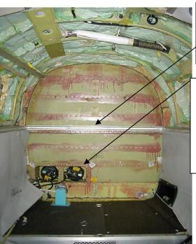
Remove this extruded upholstery rail if it covers the lower row of rivets in the lap joint. This will enable inspection for cracks along the rivet line.
